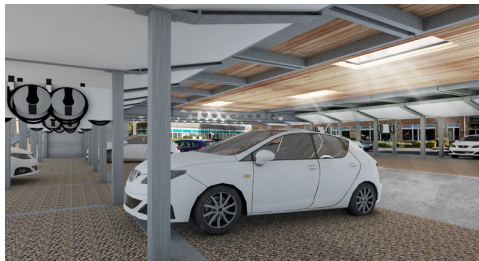
Electric vehicle charging points in line with SHS columns. One charge point for each parking bay.
